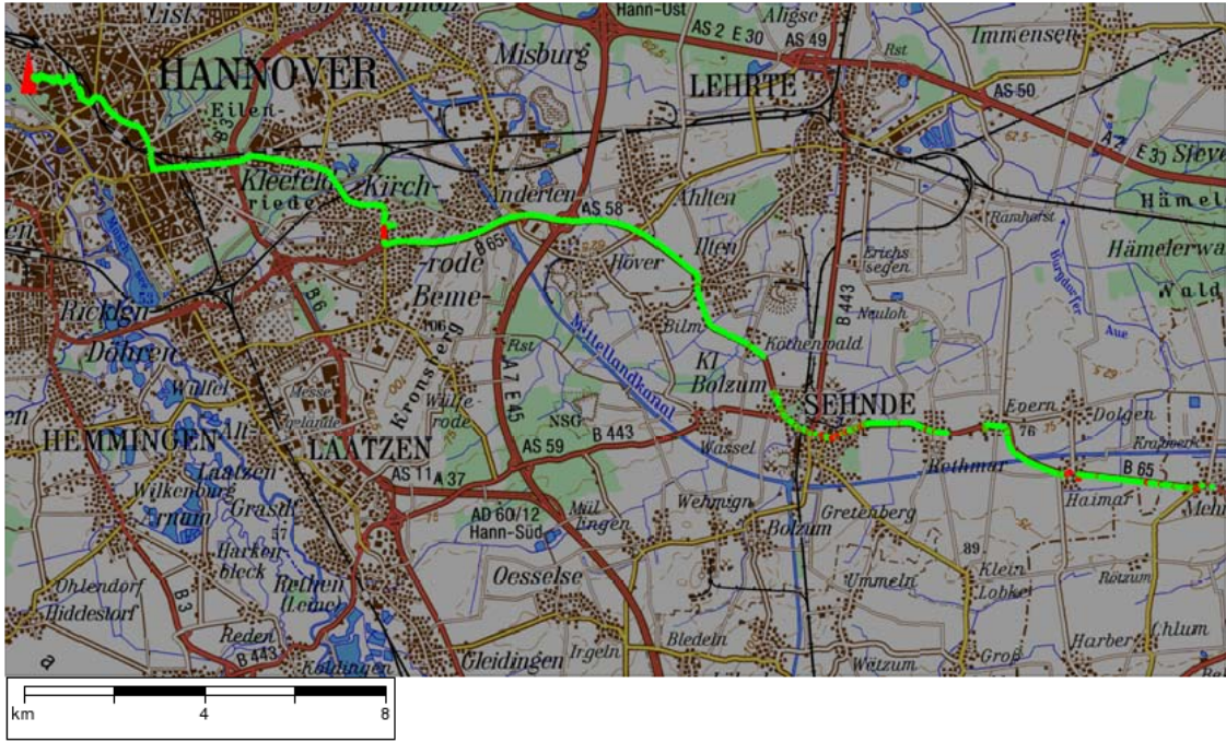
Figure 13: Measurement of the coverage limit in 4 QAM Mode (Coderate: 0.33), green: audioframes ok, red: one or more audioframes corrupted (mapsource: Bundesamt für Kartographie und Geodäsie)
