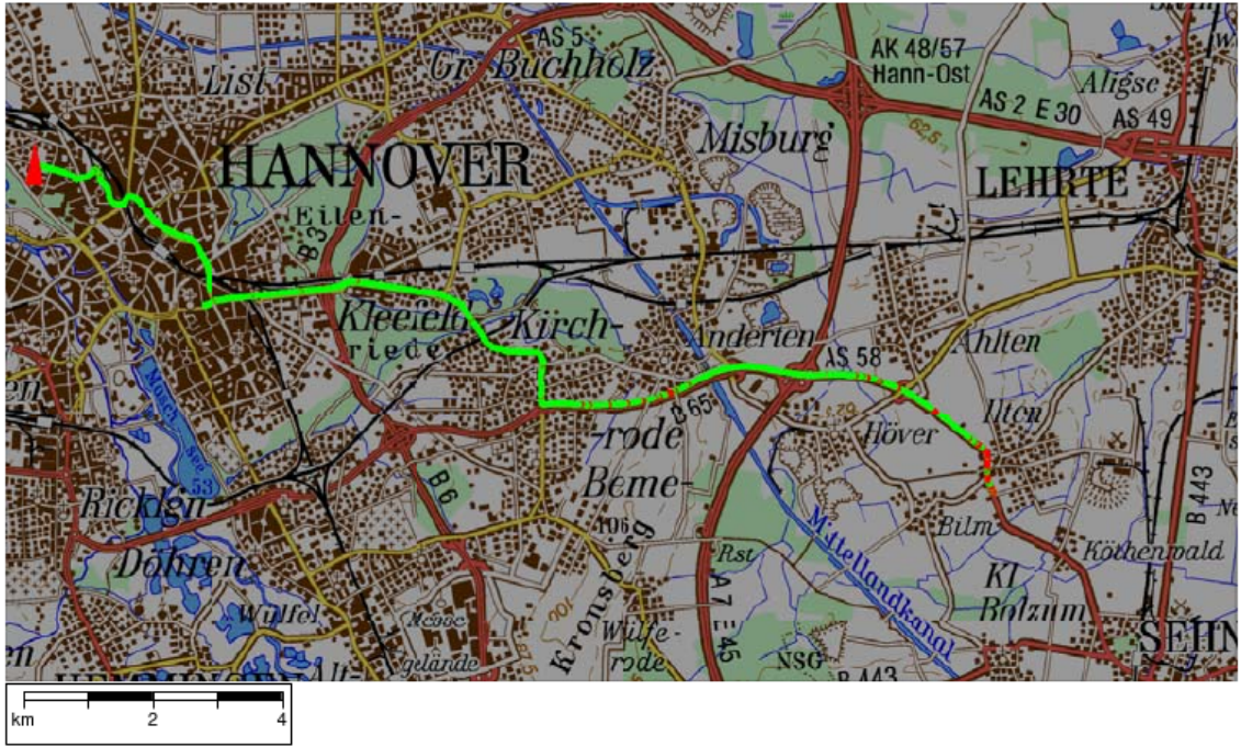
Figure 16: Measurement of the coverage limit in 16 QAM Mode (Coderate: 0.5), green: audioframes ok, red: one or more audioframes corrupted (mapsource: Bundesamt für Kartographie und Geodäsie)
